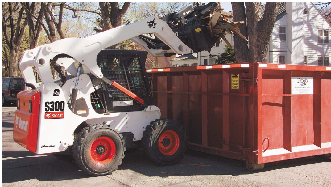
Large-frame, vertical-lift-path loaders in the new K-Series (S250, S300, T300 and A300) have an additional 2 inches of lift height. This added capability assists in loading over high-sided containers and trucks.
