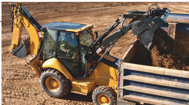
An E-Series loader feature that both operators mentioned is the machine's ability to quickly raise the boom without having to neutralize the transmission in short-cycle operations.
