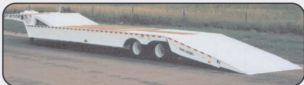
TE70HT - Ground and dock loading capabilities.
