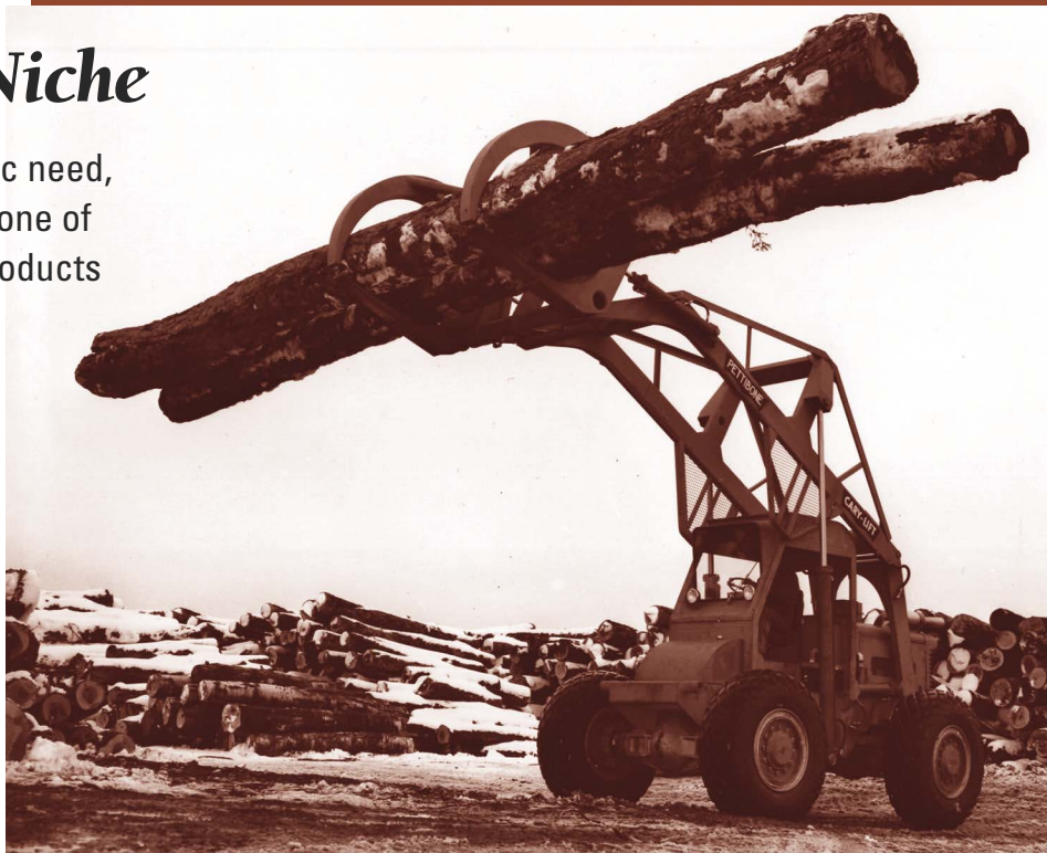
Pettibone's Model 54 Cary-Lift has a lift capacity of 10,000 pounds. Cary-Lifts have been in production since the early 1950s.
